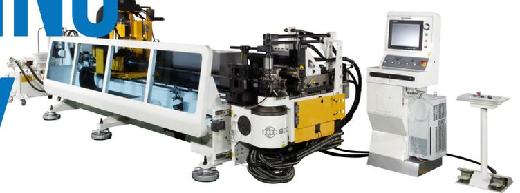
Langbow offer a wide range of new tube bending machines from Soco ranging from NC machines to multi axis CNC tube bending machines and automatic load and unload production cells. Langbow also provide Soco all electric machines and the versatile left and right hand bend head machine in both 32 mm and 52 mm capacity versions for more complex shapes and variable radius bending. Click on any of the tube bending machines below for full specifications.
